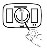
Open battery compartment with a coin.
